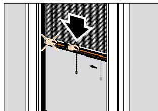
**Disengaging the Rollo insect protection screen**
